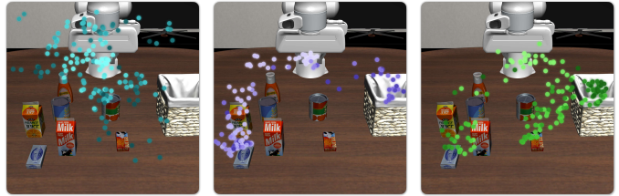
Fig. 12: Comparison of exploration behaviors on the task, "pick up the butter and put it in the basket" for RLPD (left), DSRL (center), and TMRL (right). While RLPD explores via random action noise and DSRL relies on action samples from the conditional distribution, TMRL leverages action sequences from smoothed contexts, resulting in broadened, yet coherent exploration.
